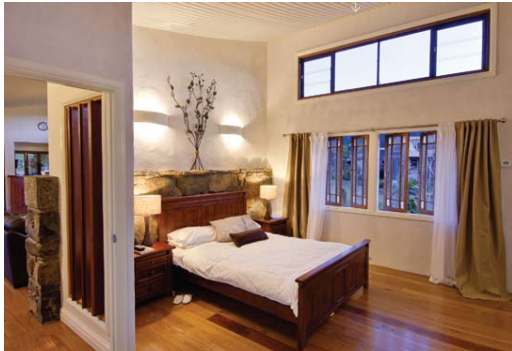
Beautiful “organic” walls include locally quarried rock, and clay and straw render over bamboo lath
